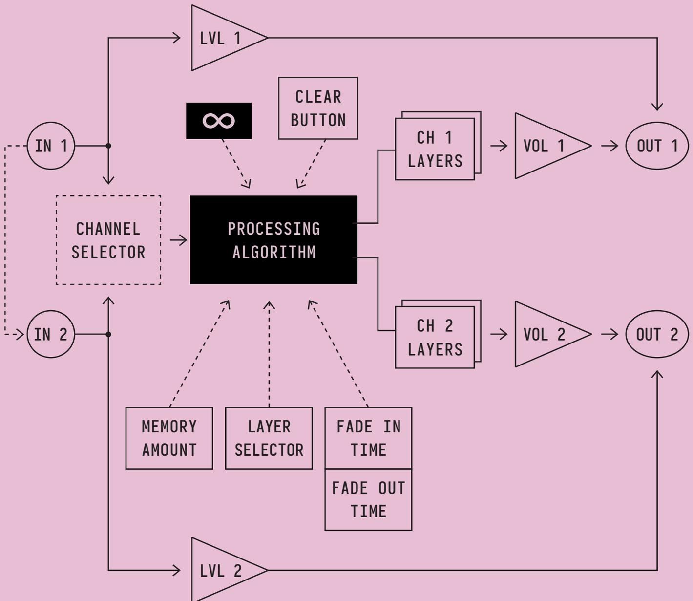
Starting from the hardware revision 1.3 (see the back of the module) **IN 1** is normalized to **IN 2** - if a cable is not plugged into **IN 2**, signal from the **IN 1** will be used instead.
